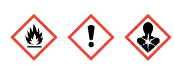
Extremely flammable liquid and vapour. Suspected of causing cancer. Causes serious eye irritation. May cause respiratory irritation.
